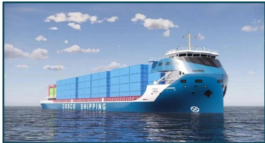
The first All-electric 700 TEU container ship, 119.8 meters LOA, beam of 23.6 meters and a designed draft of 5.5 meters. (26 th July 2023)
