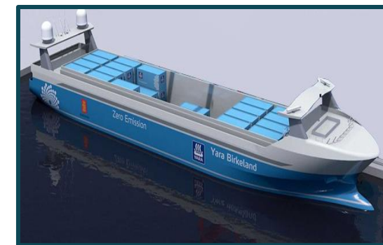
80m long with a beam of 14.8m and a depth of 12m 120 TEU Capacity - Zero Crew.
